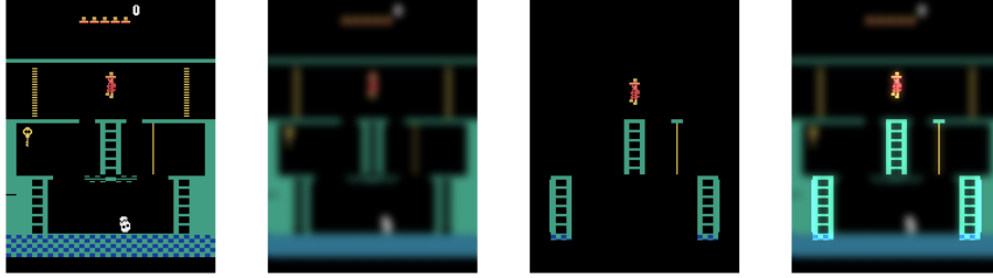
Figure 2: Saliency Map Generation. We produce heat maps for the model based on a pseudo random interval to authentically simulate a human in the training loop. A Gaussian filter with blur radius of 3 is applied to the observation image. The resulting vector is added to the template mask. The final saliency map is depicted in the far right image of the figure.
